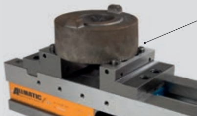
clamping unmachined parts round
