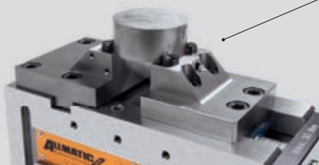
clamping unmachined parts round
